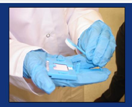
Fold the device at the hinge joint.
