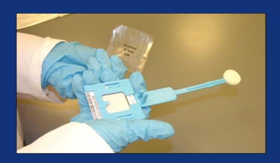
REMOVE the plastic protective film from the FTA card holder.
