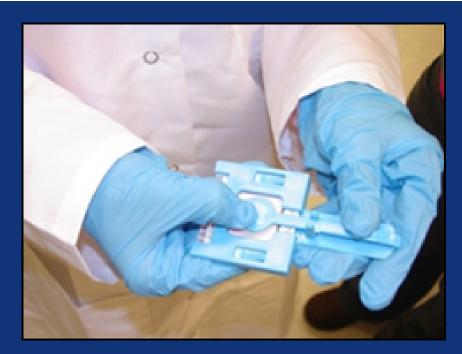
Press the foam applicator onto the FTA card and snap down two notches to the LOWEST position on the stem snap located on the handle. Ensure that there is contact between the foam head and the FTA card.
